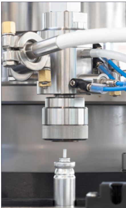
1 st green gas filling machine for pMDIs for new generation green propel- lants (HFA 152a & HFO 1234ze)
